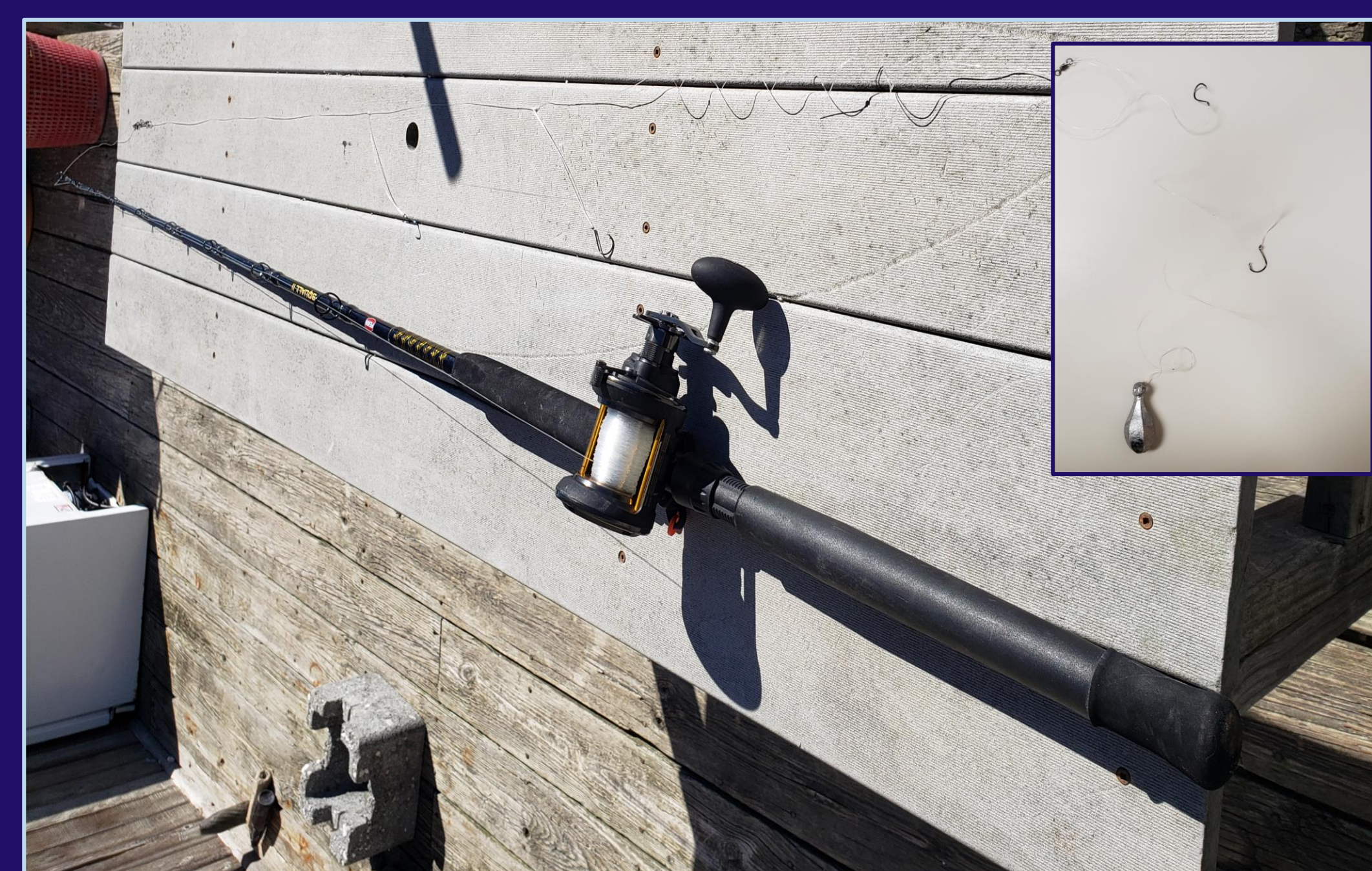
Figure 6: Set-up of hook-and-line rig. Two hooks are placed 12" apart and weighed down with either 8, 10, or 12 oz. sinker weights
