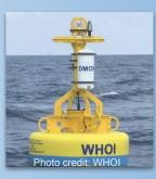
Digital Acoustic Monitoring "DMON" Buoy
